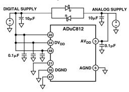
Figure 43. External Dual-Supply Connections
